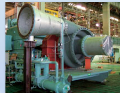
Gas blower for Acrylic Acid plant
