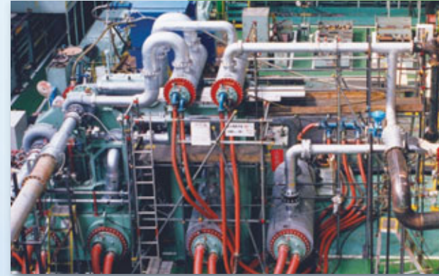
Nitrogen gas compressor (Combined type) for Air separation plant
