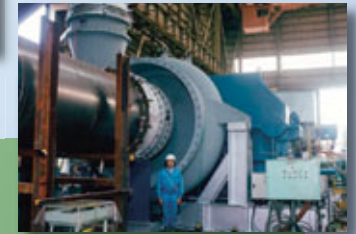
Gas and Air compressor (Combined type) for Styrene plant
