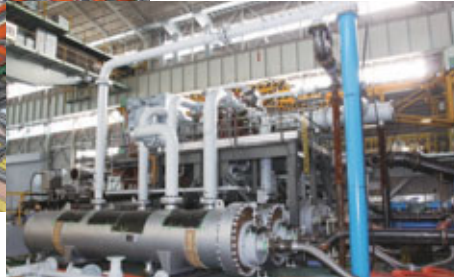
Booster Air Compressor Module for Air separation plant
