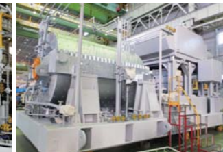
Main Refrigerant Compressor for LNG Plant
