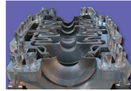
Fabricated Casing for horizontally split type
